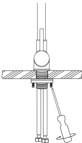
Tighten the mounting nut with the screws until faucet is firmly secure.
