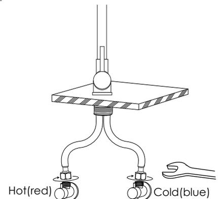
Connect hot and cold water lines to the inlet pipe and tighten with a wrench until snug. Do not over tight.
