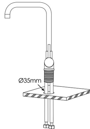
Ensure there is a Ø35mm through-hole on the counter. Position and insert faucet into faucet countertop hole.
