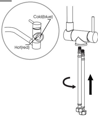
Manually connect the supply hoses, ensuring the red mark aligns with hot water hose and the blue mark aligns with cold water hose.
