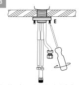
Position faucet on the installation surface. Fit flexible hoses through hole on countertop or sink.
