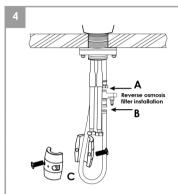
(A) Attach RO Connector to inlet port. Ensure gasket is present.
