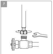
Connect hot and cold water lines to the inlet pipe and tighten with a wrench until snug. Do not over tight.
