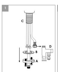
Remove the mounting nut (A) and washer (B) from the threaded shroud (C) Remove RO Connector (D)
