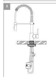
Secure weight on lowest vertical point on pull-out hose side. (not on quick connect side)
