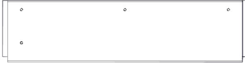
D02 FAN FRAME - W4L18915 (x1) 1 7/16"x5 1/4"x20 13/16" (36x134x529)
