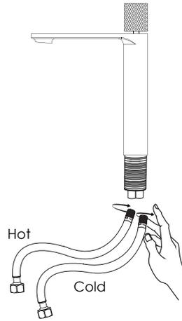
Install hot and cold water lines to the faucet. Hand tight hoses firmly.
