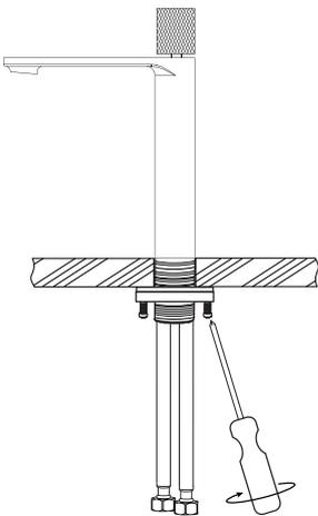
Tighten the mounting nut with the screws until faucet is firmly secure.
