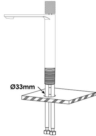
Ensure there is a Ø33mm through-hole on the counter. Position and insert faucet into faucet countertop hole.
