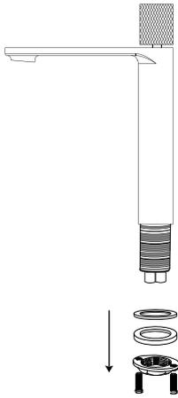
Remove the washer and mounting nut.
