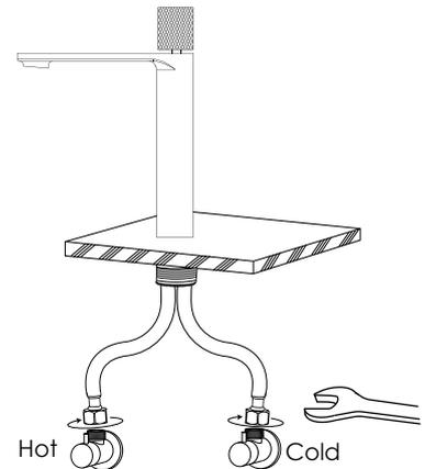
Connect hot and cold water lines to the inlet pipe and tighten with a wrench until snug. Do not over tight.
