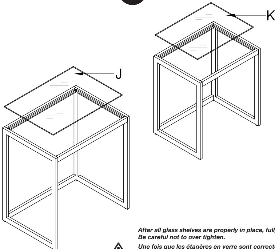
*After all glass shelves are properly in place, fully tighten all screws.
