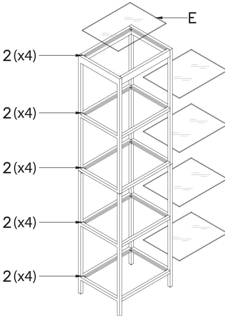
*Once all shelves are in place, then fully tighten screws. You may need to slightly loosen screws and retighten again after standing upright to ensure a stable and level book shelf.*
