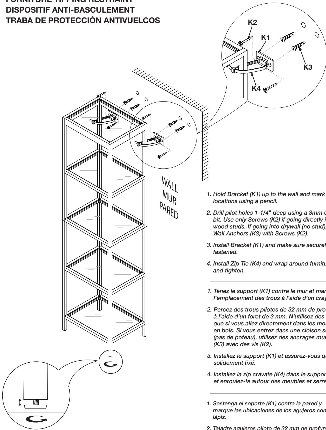
**NOTE:** Use the leveling feet to make sure furniture is level on the floor before using.
