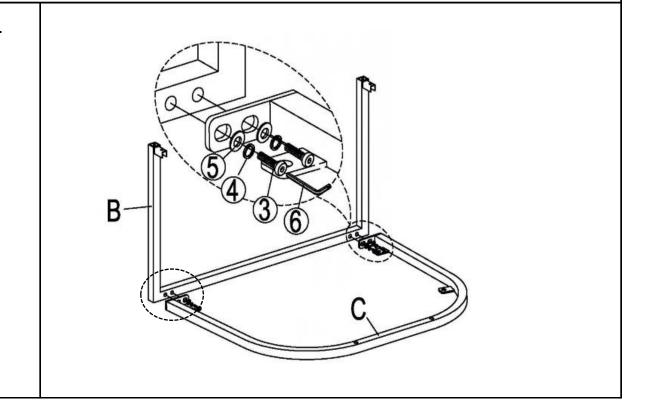
Attached Support metal tube (B) to Support rail (C) using Bolts(3), Washers(4), and Spring Washer(5) with Allen Key(6) as shown in above picture.
