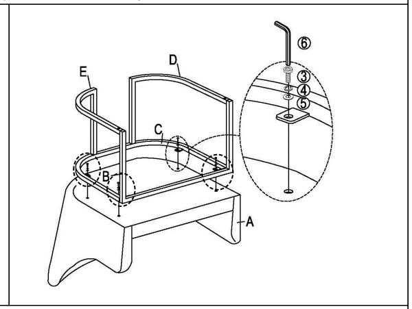
Attached Support metal tube (B), Support rail (C), Left side tube (with Pre-attached Leveller) (D) and Right side tube (with Pre-attached Leveller) (E) to Backrest (A) using Bolts(③), Washers(④), and Spring Washer(⑤) with Allen Key(⑥) as shown in above picture.
