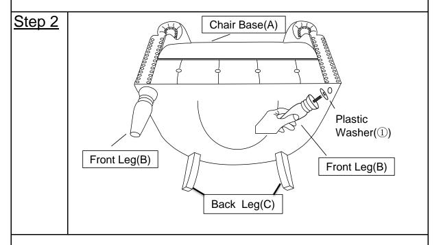
Install the Front Leg(B) into the bottom of the Chair Base(A) by placing the Plastic Washer(①) onto the threaded stem.
