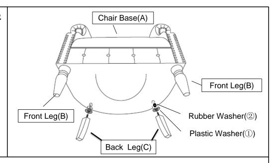
Install the Back Leg(C) into the bottom of the Chair Base(A) by placing the Plastic Washer(①) and Rubber Washer(②)onto the threaded stem.
