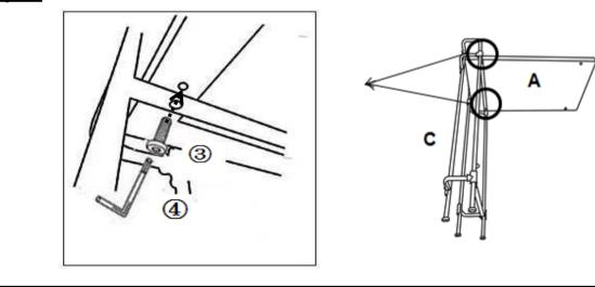
Open the carton and place all parts onto a clean, non-marring surface. Place the Right Leg Frame(C) on it's side as shown. Attach the top Wooden Tray(A) to the Right Leg Frame(C) using Bolts(③) with Allen Key(④). **Do not fully tighten the Bolts.**
