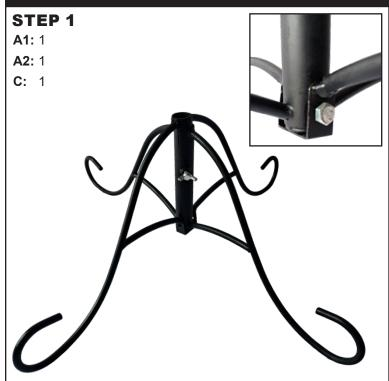
Remove Bolt and Nut (C) from Inner Leg Base (A1).
