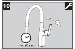
Before connecting supply lines to the water valves, flush each water valve to remove dirt and particles that can affect the functioning of the faucet and void warranty.
