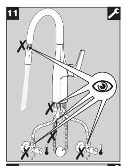
Double check all connections for leaks.
