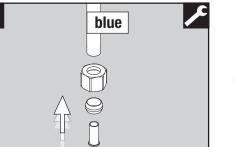
Slide the nut and the ring over **the blue hose**, then push the grommet into the hose.
