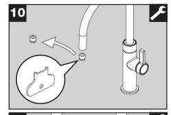
Remove aerator (5) using the aerator key (6).
