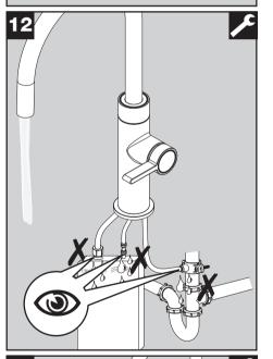
Double check all connections for leaks.
