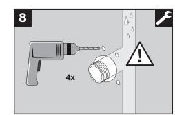
Drill 3/32" (2.5 mm) holes where marked. If using the provided anchors, drill 1/4" (6 mm) holes.
