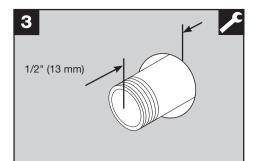
Make sure the threaded pipe has a 1/2" IPS thread (1/2" - 14NPSM, Length 1/2"/13 mm)
