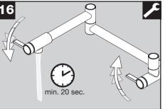
Turn on water supplies. Open the water valves and flush for at least 20 seconds the lines and the faucet.
