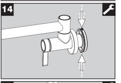
Tighten set screws in the wall flange with allen key 3/32" (2.5 mm).
