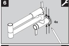
Mark the screw holes in the wall flange.
