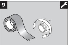
Seal the thread with thread sealing tape or hemp.
