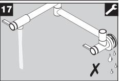
Check connection for leaks. Re-tighten if necessary, but do not overtighten.
