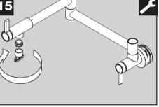
Remove aerator (3) using the provided key (4).
