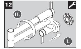
Thread faucet onto pipe. Tighten securely, but do not overtighten.
