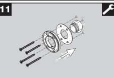
Install the gasket and the wall flange using the 4 screws (and anchors if required) provided.
