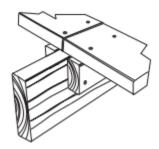
Maintain a 1/4" (0.64 cm) distance between all decking material and any permanent structure or post. After all decking has been attached, snap a chalk line (white or yellow chalk recommended) flush with or up to 1-1/2" (3.81 cm) out from the deck framing and trim with a circular saw. Composite decking requires proper ventilation and drainage to ensure longevity.
