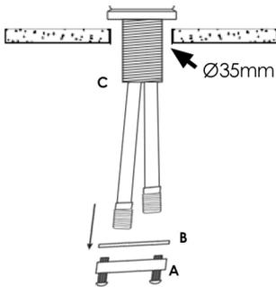
Ensure there is a Ø35mm through-hole on the kitchen counter. Remove the mounting nut (A) and washer (B) from the threaded shroud (C).
