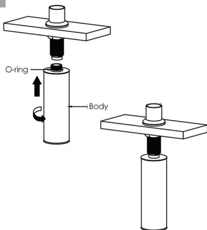
Hand secure body tank to connector rod.
