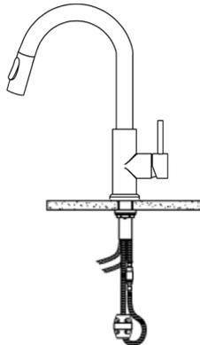
Secure weight on lowest vertical point on pull-out hose side. (not on quick connect side)
