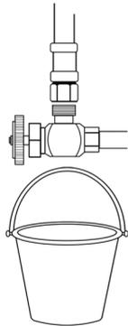
Before connecting supply hose, flush supply valves to clear any debris. Place a bucket underneath valves and run water for 5 to 10 seconds. Turn water off.
