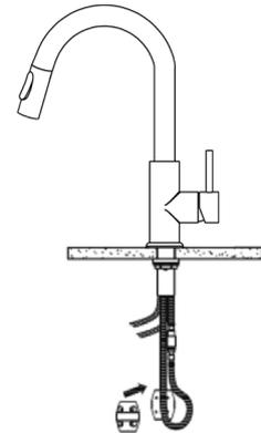
Connect pullout hose to quick connect and insert weight (loose-install)
