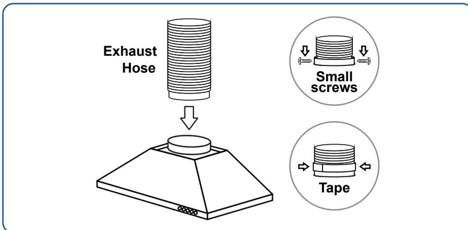
24. Connect and route the exhaust pipe to the exterior of the house for ventilation.
