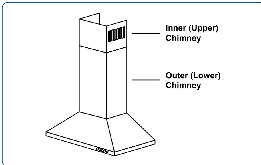
3. Attach the lower chimney bracket to the lower chimney.
