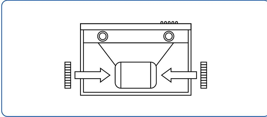
26. Re-insert either the mesh or baffle filters into the range hood.
