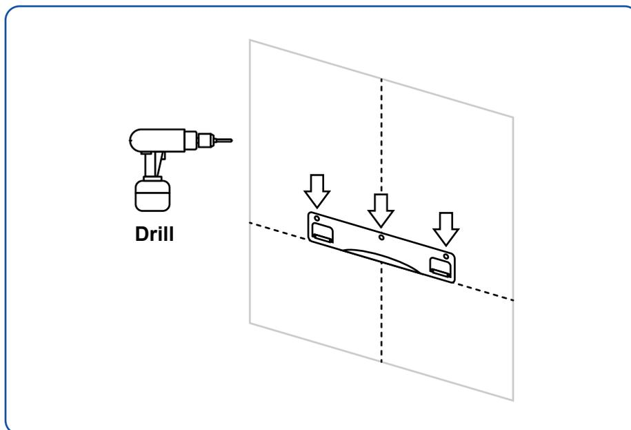
12. If mounting directly to a wood stud, use the (3) provided ST 4x30 mounting screws to secure the mounting bracket in place by drilling (3) pilot holes.
