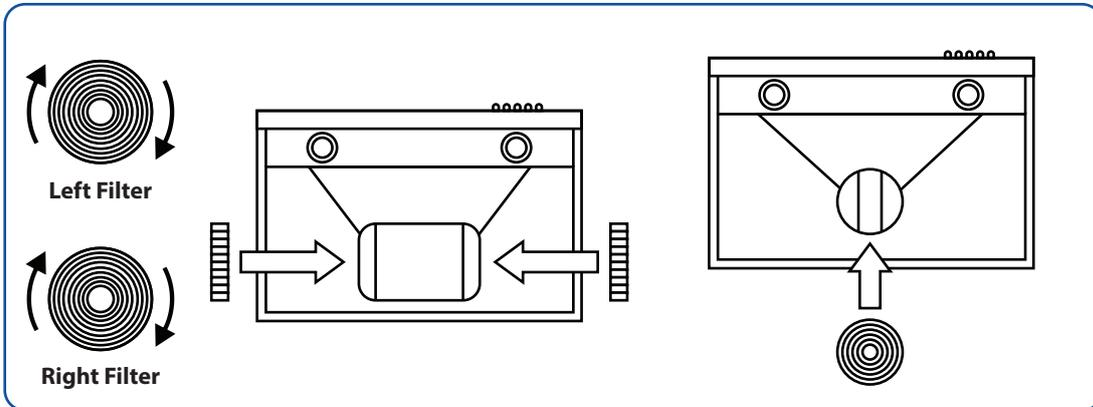
4. To replace the filter, rotate it counterclockwise and then remove it. After that, install the new charcoal filter and twist it clockwise to lock it in place.
