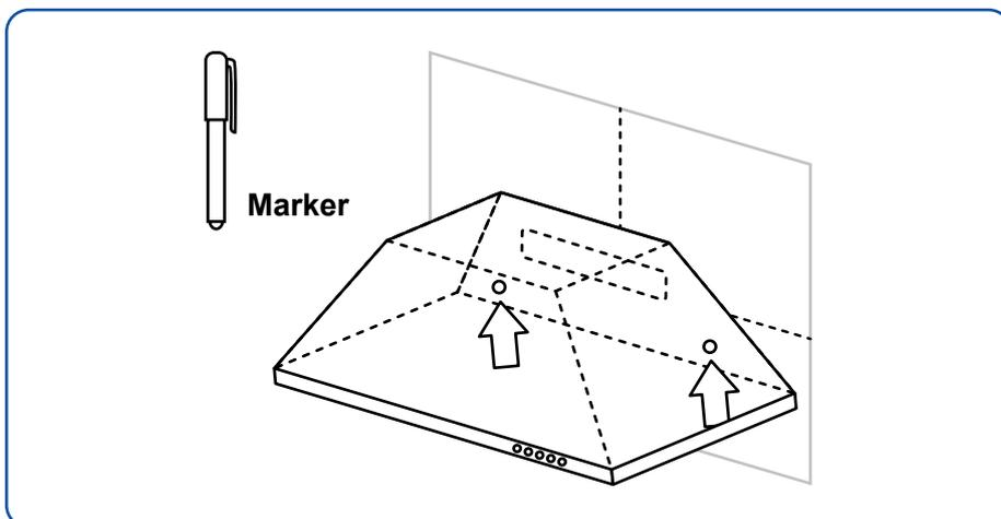
17. Use a drill to make two holes in the wall at the marked locations. For wood, use a 5/32" drill bit, and for wall anchors, use a 5/16" drill bit.
