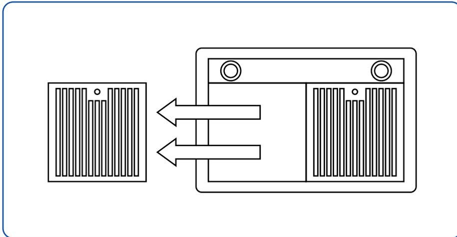
16. At the back of the range hood, there will be 2 visible holes. Mark their position on the wall and remove the range hood from the mounting bracket.
