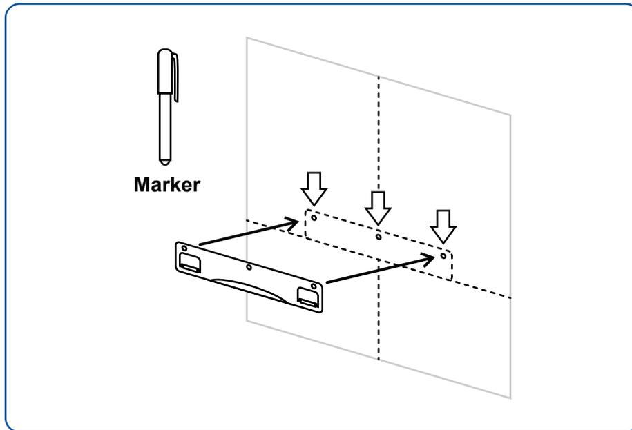
11. Use a drill to make three holes in the wall at the marked locations. For wood, use a 5/32" drill bit, and for wall anchors, use a 5/16" drill bit.
