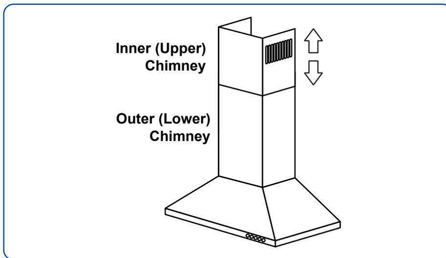
12. Lift the upper chimney to the ceiling and mark on the wall the position of the upper chimney mounting bracket. Make sure that the markings align with the centerline that was previously marked.
