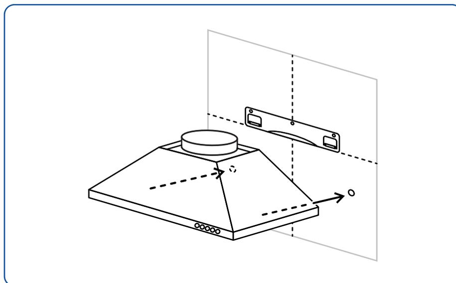
19. Fasten the range hood using (2) ST 4x30 screws.
