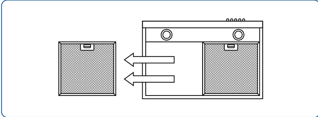
2. The placement of the charcoal filter varies depending on the model. In some models that only require 1 charcoal filter, the opening is in the middle of the motor. For models that require 2 charcoal filters, the openings are positioned on the sides of the motor. If you have any inquiries regarding the specific model that you have purchased, please don't hesitate to contact our support team.
