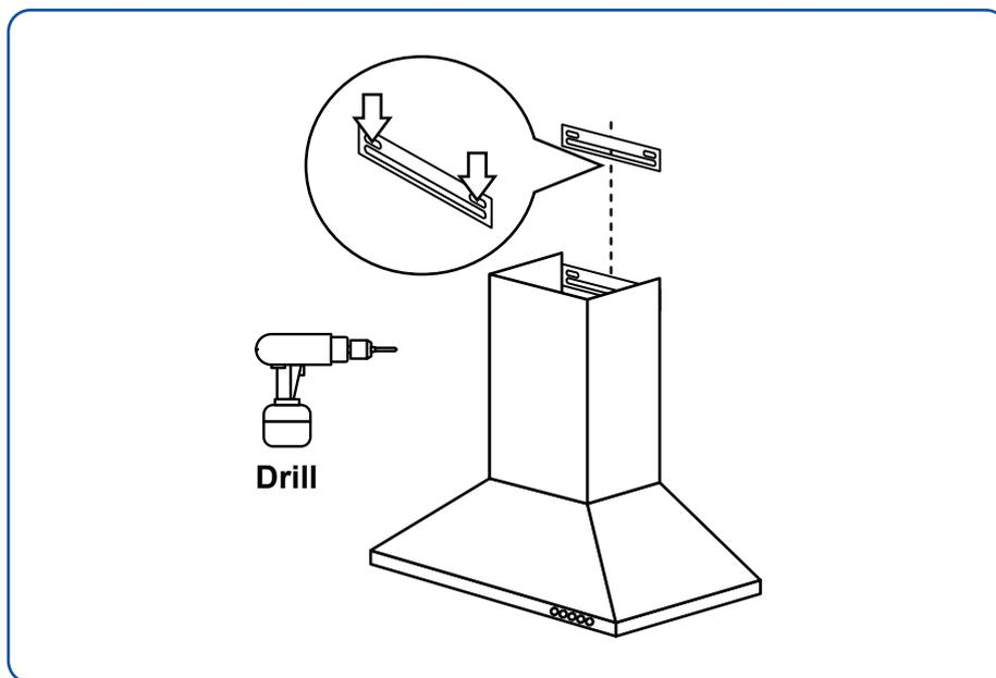
15. If mounting directly to a wood stud, use the (2) provided ST 4x30 mounting screws to secure the mounting bracket in place by drilling (2) pilot holes.
