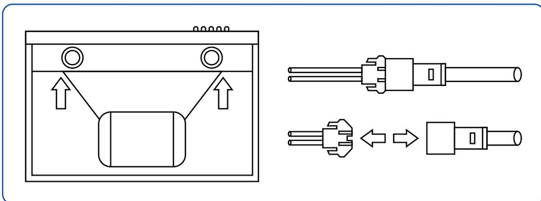
5. Take out the LED light by pressing the long silver bar that covers the LED. Push the LED outwards and downwards.
