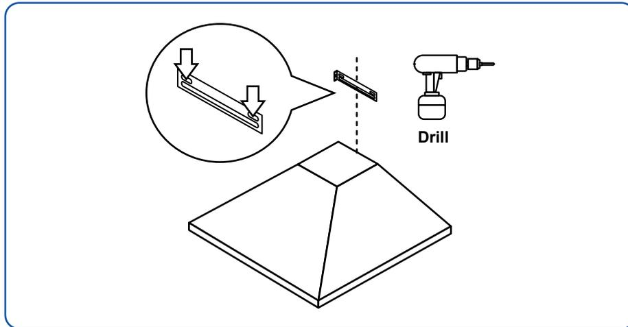
8. If mounting directly to a wood stud, use the (2) provided ST 4x30 mounting screws to secure the mounting bracket in place by drilling (2) pilot holes.
