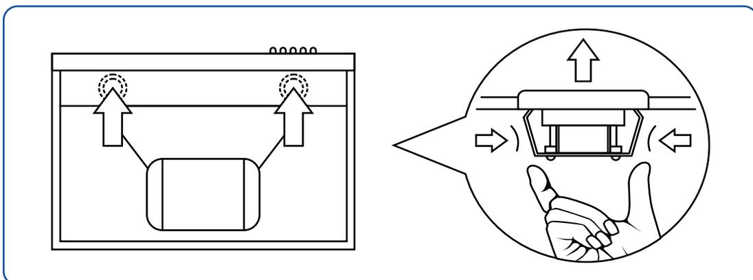
6. Insert the new LED lights into the opening inwards and upwards and apply gentle pressure until you hear a click and feel the light sitting securely in place.
