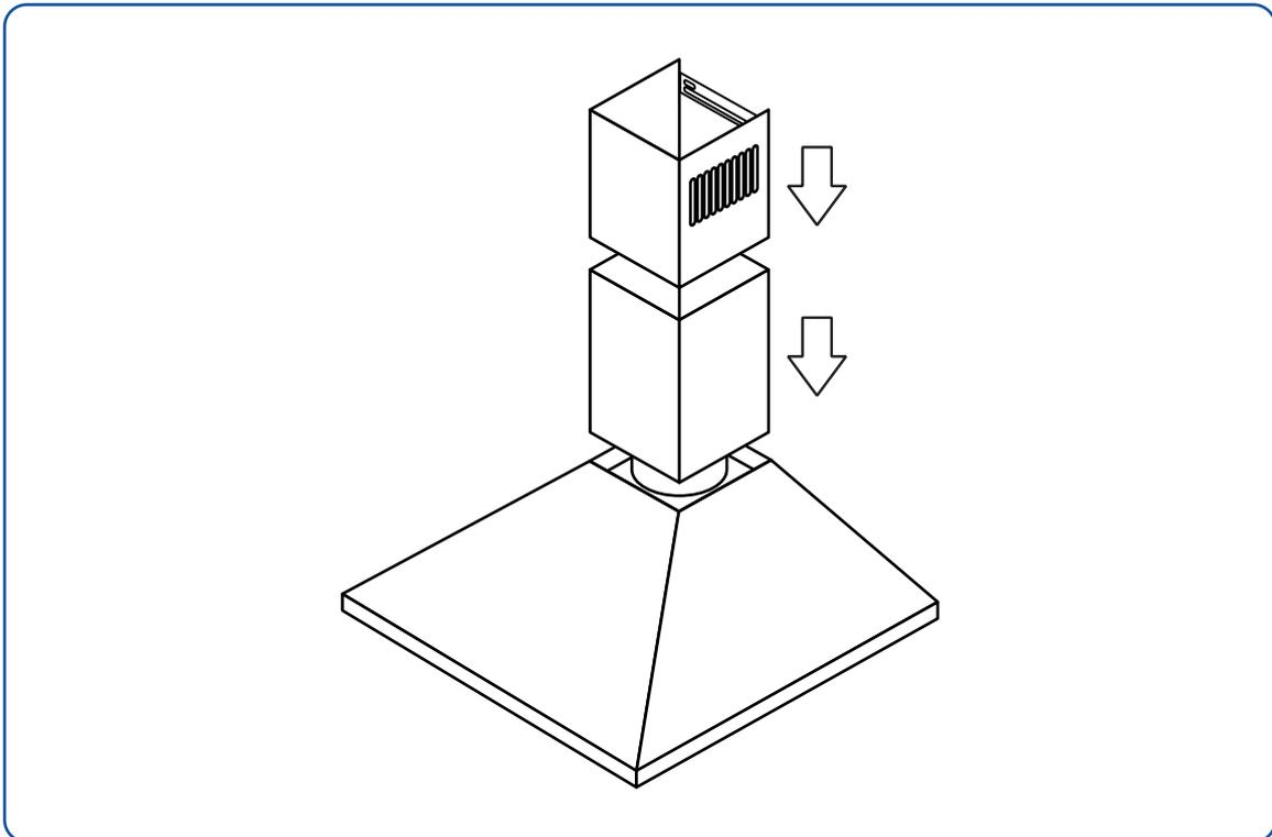
17. To attach the upper chimney, lift it onto the upper support bracket and use one ST 4x10 screw on each side of the chimney to secure in place.
