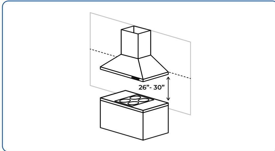
2. Once the ideal mounting height is determined, create a marking at a horizontal level. This will be the bottom of the range hood.
