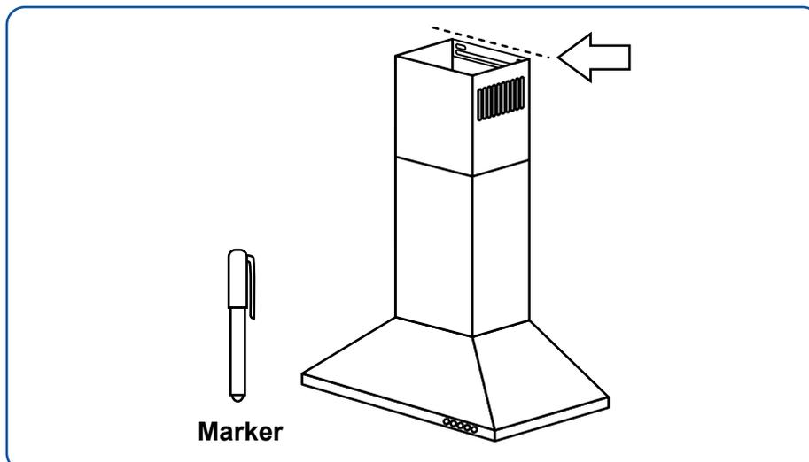
**When venting through the wall, please note that it is NOT required for the chimney to make contact with the ceiling.**
