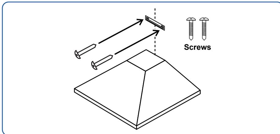
9. If mounting to the wall, use the (2) provided wall anchors prior to installing the (2) ST 4x30 mounting screws. Insert the plastic wall anchors firmly into the drilled holes.
