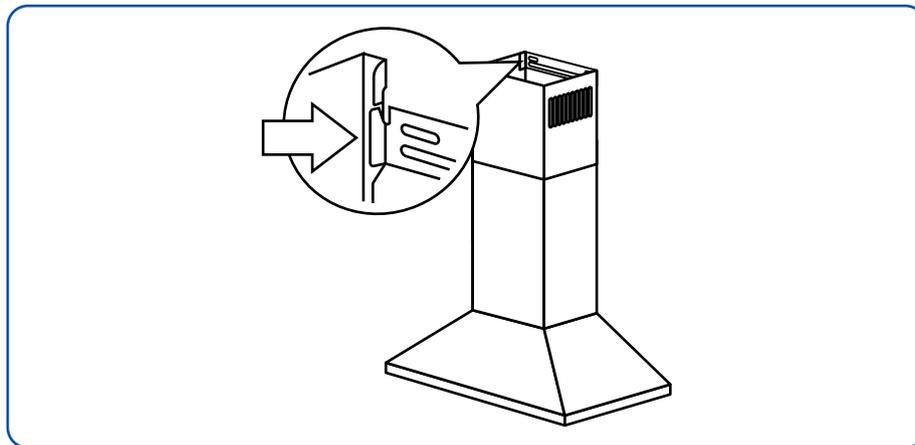
19. Some range hood models may be equipped with screw holes at the bottom of the lower chimney. Use (2) [1 on each side] 4x10 mm screws to tighten and secure.
