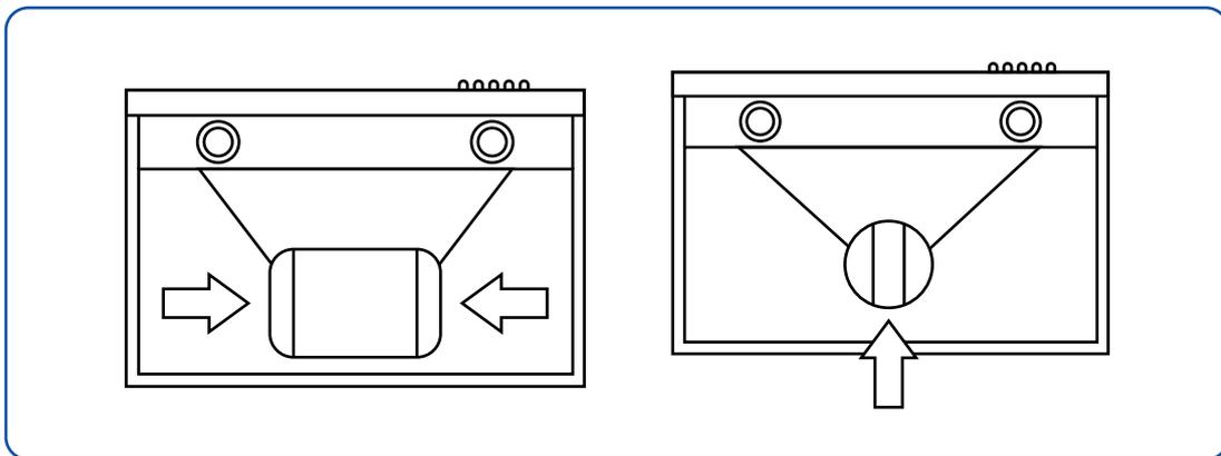
3. Take one filter and attach it to the motor. Rotate and twist it clockwise until it locks in place. If your range hood model calls for two filters to be installed, then the filters should be installed on each side. Repeat the previous step by taking another charcoal filter and attaching it to the other side of the motor. Rotate and twist it clockwise until it locks in place.
