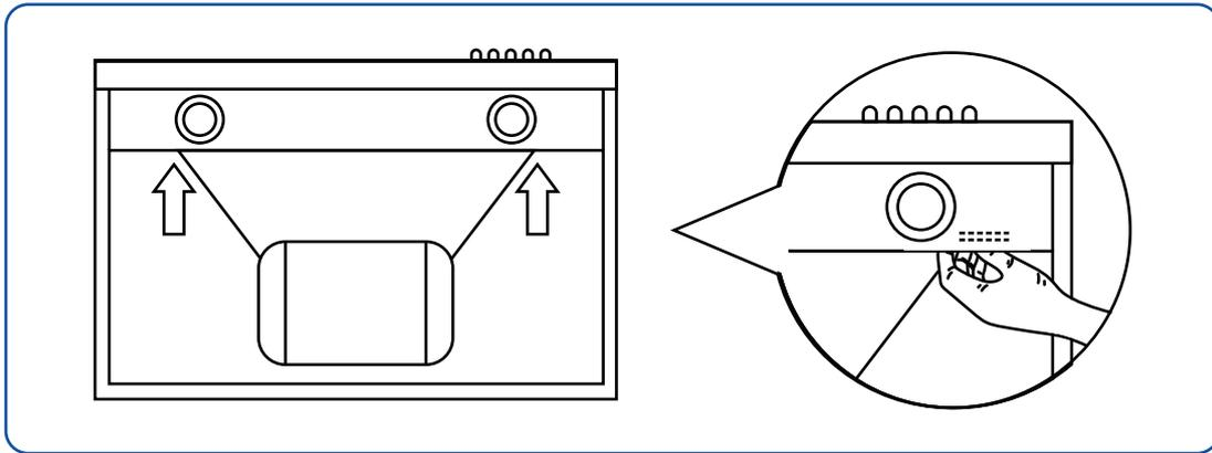
4. The wires for the LED lights are connected using a snap-down connector. To disconnect the LED lights, press down on the connector and gently pull the opposing electrical wire away from the connector.
