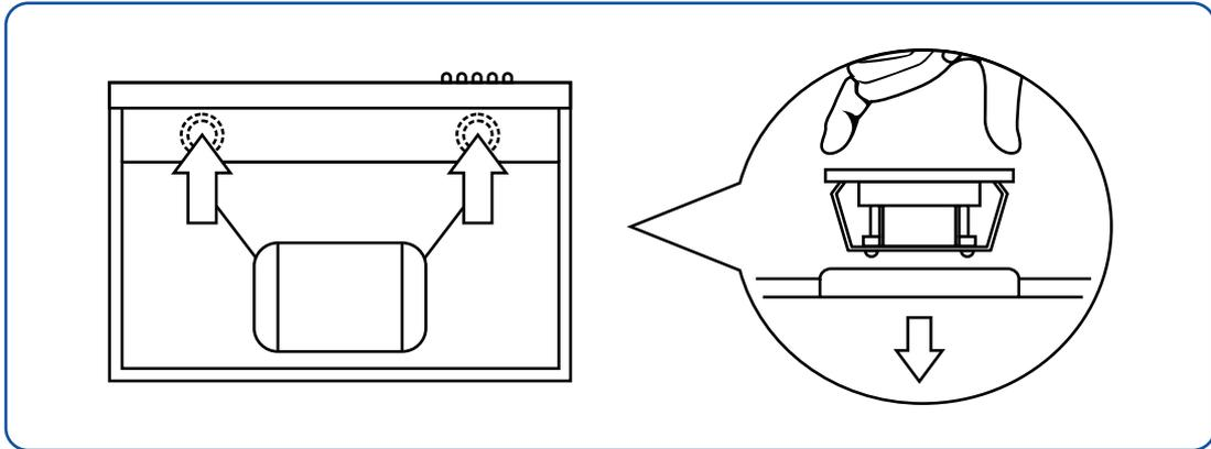
7. Reconnect the electrical wiring in the range hood with the LED snap connector.
