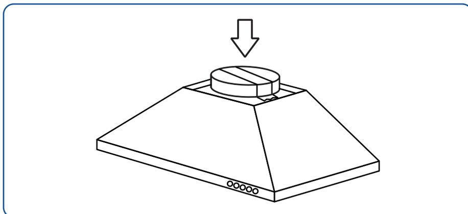
22. Ensure that the damper is correctly installed. Attach the vent flaps in the exhaust port on the top of the range hood. Check to make sure that the flaps can open smoothly and without any obstructions. Please note that the bumps on the flaps should face upwards and outwards.
