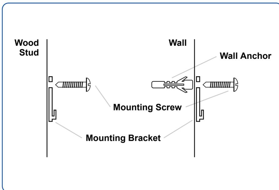
14. Mount the range hood onto the mounting bracket.
