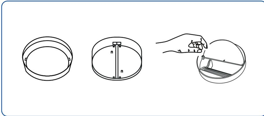
23. Attach a 6-inch round aluminum duct exhaust hose to the round vent air flap and secure it with two small screws, as well as tape or a hose clamp with tape.
