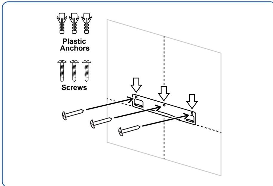
13. Secure the mounting bracket with the selected method of choice.
