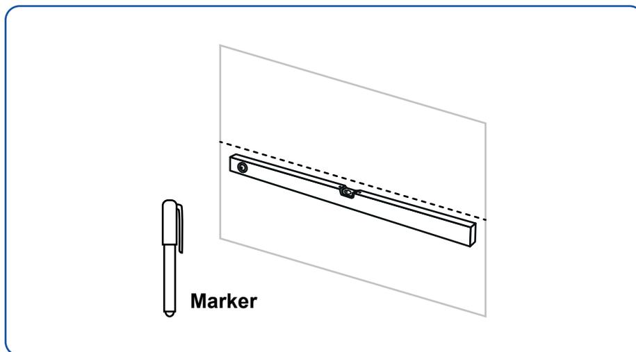
3. Locate the vertical centerline on the wall in reference to the horizontal line, marking the position where the range hood will be mounted. This line will reflect the center point.
