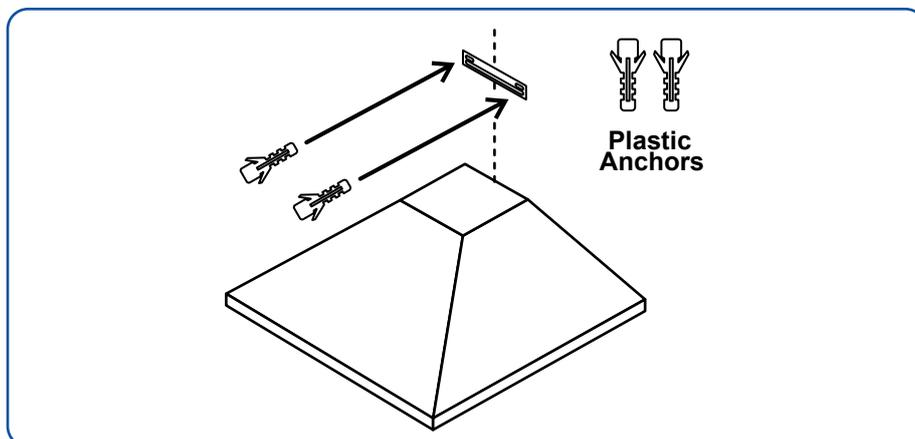
10. Attach the upper chimney bracket to the upper chimney.
