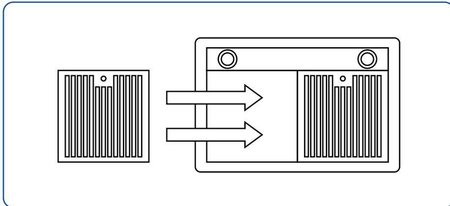
21. Remove the protective tape from the damper.
