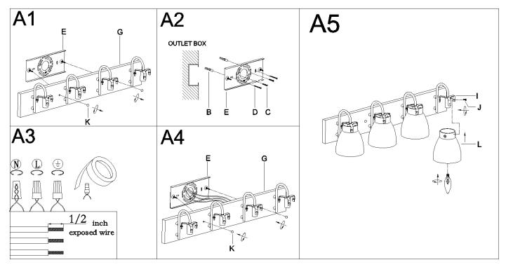
Step A1 » Unscrew knob nuts (K) from back plate (G) then gently remove mounting plate (E). Then set them aside for later installation.
