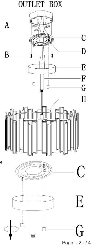
3 » Pass the fixture wires through tube (F) and canopy (E), then screw tube (F) and canopy (E) onto the top of fixture body (H).
