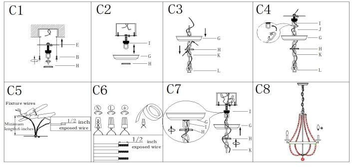
Step C1: .Attach the single bar (E) to outlet box with mounting screws (B). The side of single bar marked "GND" must face out Step C2: Pass canopy (H) over the mounted collar loop (I) then secure with threaded ring (H) to test the height .Unscrew
