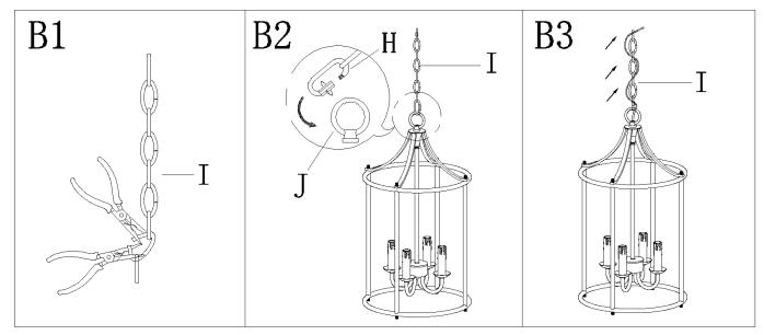
Step B1: By measuring, determine the correct number of links needed for proper hanging height. Using the chain pliers, disconnect and discard the remaining chain.
