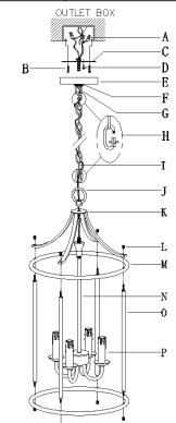
Step A1: Fix the iron ring (M) on the tube (O) with knob nut (L).
