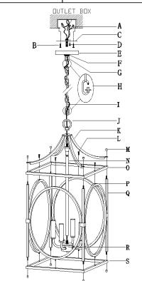
Step A1: Slip stem (N) over the wires and then thread it into the top of fixture loop assembly (R).
