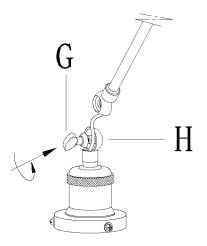
2) Carefully and gently pull the wires and fiberglass sleeve from the another end of arm(I) ,meanwhile push the socket (J) till two parts of joint are close each other , lay wires in the cave of joint(H), then proceed to push till the two parts are put together, secure with the stud
