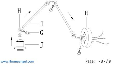
3) Connect the black and white wires found in the plate (E) to the wires with plug found inside the accessories bag. Secure the connections with plastic wire connectors.
