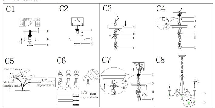
Step C1: .Attach the single bar (E) to outlet box with mounting screws (B). The side of single bar marked "GND" must face out
