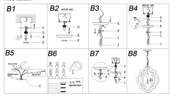
Step B1: Remove the threaded ring (F) from collar loop(G). Attach the single bar (C) to outlet box with mounting screws (B). The side of single bar marked "GND" must face out, Unscrew the collar ring (H) from the collar loop.
