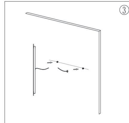
Connect the mirror wires with your main wires and hang the mounting hole to the screw on the wall.
