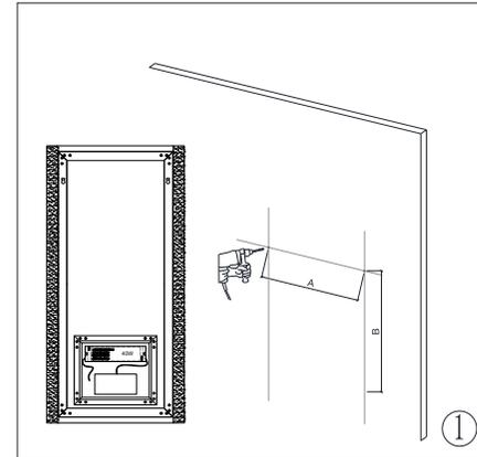
Measure the distance of the mounting hole, Drill holes with a suitable sized drill.
