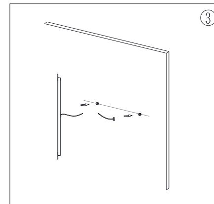
Connect the mirror wires with your main wires and
