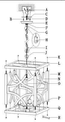
Step A1: Tighten the stem (O) onto the fixture loop assembly (P).
