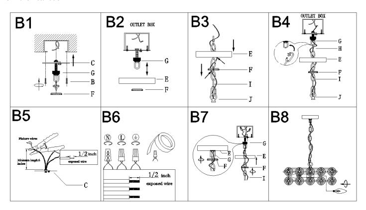
Step B1: .Remove the collar ring (F) from collar loop(G). Attach the single bar (C) to outlet box with mounting screws (B).
