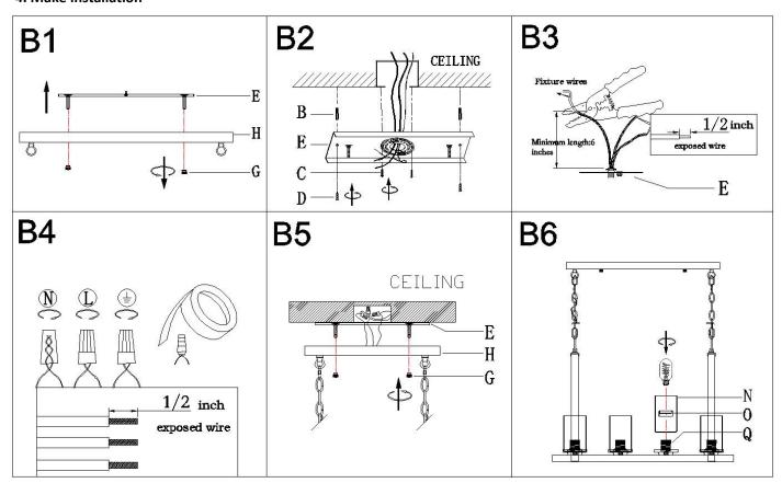
Step B1: Unscrew the ball knobs (G) from mounting plate assembly (E).
