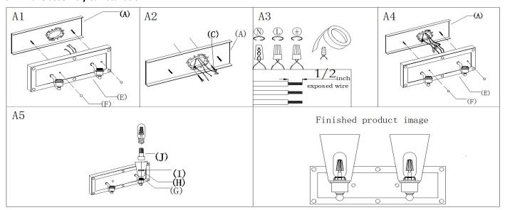
Step A1: Unscrew the ball knobs(F) from back plate(E) then gently remove mounting plate (A)
