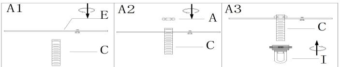
Step A1: Thread the single bar(E) onto nipple (C),
