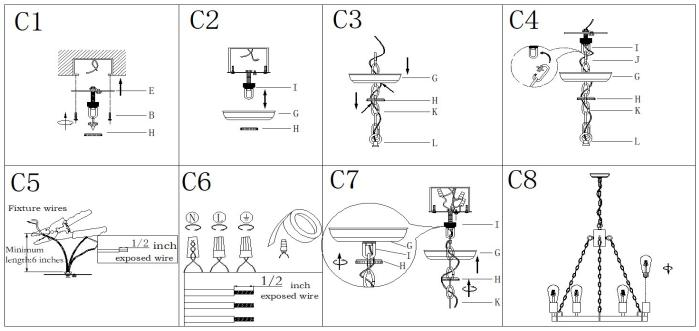
Step C1: .Attach the single bar (E) to outlet box with mounting screws (B). The side of single bar marked "GND"
