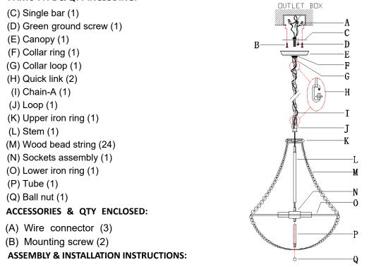
1. Carefully remove the fixture from the carton and check that all parts and accessories are included as shown in the above illustration.
