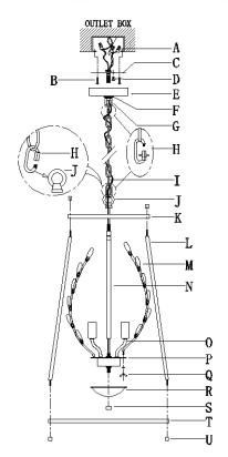
Step A1: Connect the upper iron frame (K) and lower iron frame (T) together with a tube (L) and secure with nuts (U).
