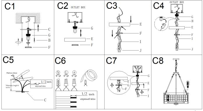
Step C1: Remove the collar ring (F) from collar loop (G). Attach the single bar (C) to outlet box with mounting screws (B). Note: the side of single bar marked "GND" must face out.
