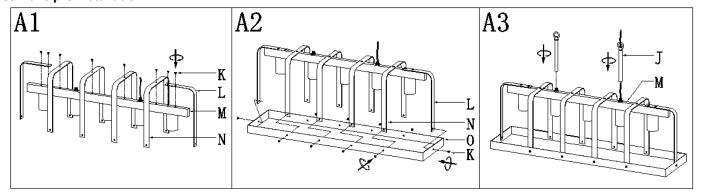
Step A1:Fix the strap iron A(L) and strap iron B(N) on the straight pipe (M) with screws (K).
