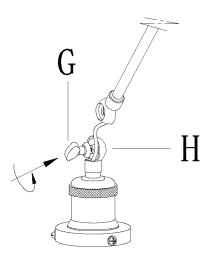
2) Carefully and gently pull the wires and fiberglass sleeve from the another end of arm(I), meanwhile push the socket (J) till two parts of joint are close each other, lay wires in the cave of joint(H), then proceed to push till the two parts are put together, secure with the stud (G). Close the arm sides together then adjust the stud again. Apply this process to the other
