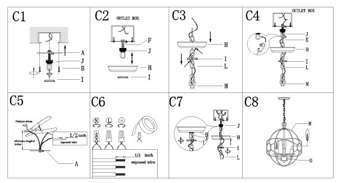
Step C1: Remove the threaded ring (I) from collar loop(J). Attach the single bar (A) to outlet box with mounting screws (B). The side of single bar marked "GND" must face out, Unscrew the collar ring (H) from the collar loop.
