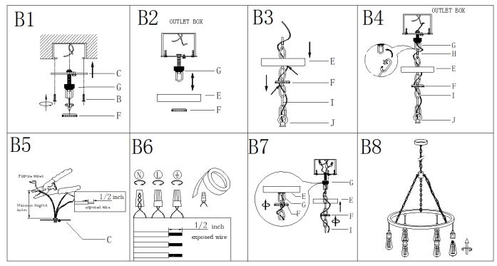
Step B1: Remove collar ring (F) from collar loop (G). Attach single bar (C) to the outlet box with mounting screws (B). Note: be sure that the side of single bar marked "GND" must face out.
