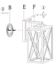
4. Carefully pass the outlet box wires through mounting plate assembly (B).
