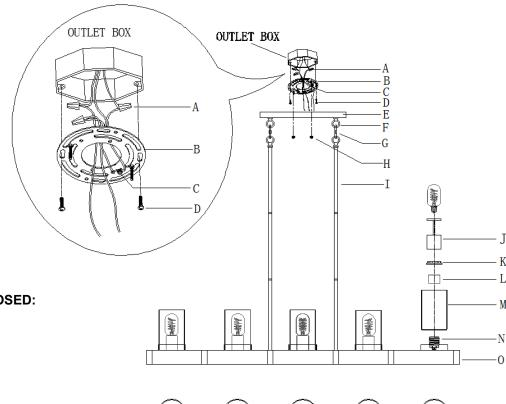
3. According your desired hanging length to select and use the tubes (I) then pass the wires through the tubes(I) to the top of loop .Gently pull wires and thread the tubes (I)onto the fixture (0) till tight
