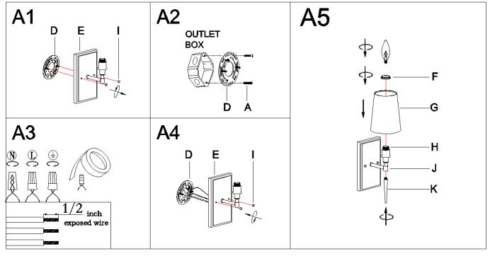
Step A1: Unscrew the ball knobs (I) from the back plate(E) then gently remove the mounting plate (D). Step A2: Secure mounting plate (D) to outlet box with mounting screws (A). Step A3: Make wire connections
