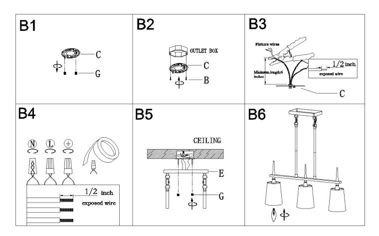
Step B1: Unscrew the knob  $\operatorname{nuts}(G)$  from round mounting plate (C) .
