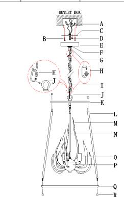
Step A1: Connect the upper iron frame (K) and lower iron frame (Q) together with a tube (L) and secure with nuts (R). Step A2: Screw the stem (N) on the fixture loop assembly (P).
