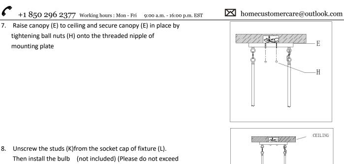
Then install the bulb (not included) (Please do not exceed the maximum capacity recommended on the socket.) Gently and carefully position glass onto the socket cap, adjust the glass to make the holes to be aligned with glass and socket cap,then secure with the studs (K) 9. Check everything is already installed properly, then you could turn on the light. Enjoy!
