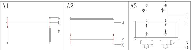
Step A1:Fasten the upper iron frame (L) and the tubes (M) together with knob nuts (K).Step A2:Fasten the lower iron frame (P) and the tubes (M) together with knob nuts (K).Step A3:Pass the wire through the upper iron frame (L),then screw the stems (J) onto the fixture loop assembly (O). Adjust the arms (N) to the proper position.
