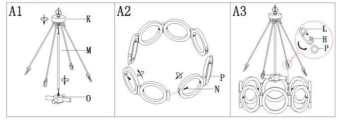
Step A1: Screw the stem (M) to the fixture loop (O), then screw the wooden columns (K) to the top of the stem (M). Step A2: Secure all wooden frames (P) together with screws (N).
