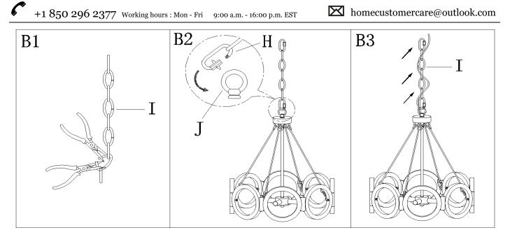
Step B1: By measuring, determine the correct number of links needed for proper hanging height. Using the chain pliers, disconnect and discard the remaining chain.
