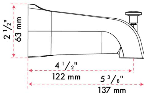
The use of copper tubing to connect the valve to the bathtub spout **IS MANDATORY**. Do not use PEX type pipes or a quick connect this could cause a flow restriction and backflow to the shower. We cannot be held responsible in the event of an incident related to an installation that does not take this advice into account.
