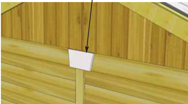
Horizontal Gable Detail Plate
