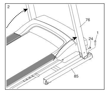
Attach the Left and Right Handrails (71, 72) to the Uprights (76) with four M10 x 45mm Screws (2); start all four Screws, and then tighten them.
