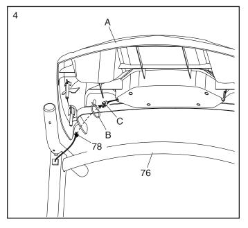
Attach the console assembly (A) to the Left and Right Handrails (71, 72) with four M4.2 x 19mm Screws (3); start all four Screws, and then tighten them. Be careful not to pinch the wires.
