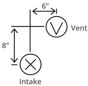
The vent termination and air intake must be in the same pressure zone and face the same direction.
